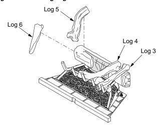
Figure 27 - Installing Logs 5 and 6
